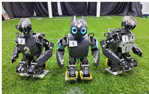
Fig. 2. ICHIRO-1 robot which is the modification of Darwin OP
