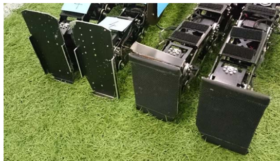
Fig. 4. The modified soles (left) and the conventional soles (right).
