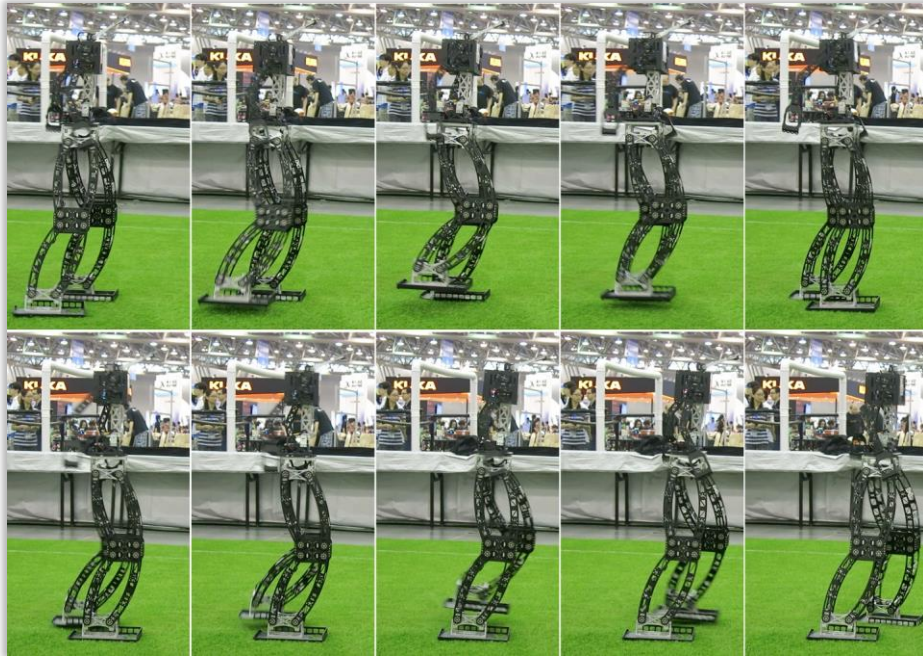
Fig. 3. Enhanced generated trajectory of Baset Adult-Size robot
