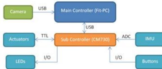
**Fig. 2.** Electronic Block Diagram
