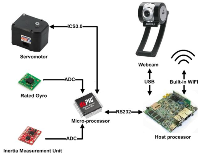
**Fig. 2.** Robo-Erectus Architecture
